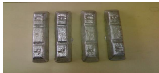
Fig 1: Ingot Structure of Al 7075
